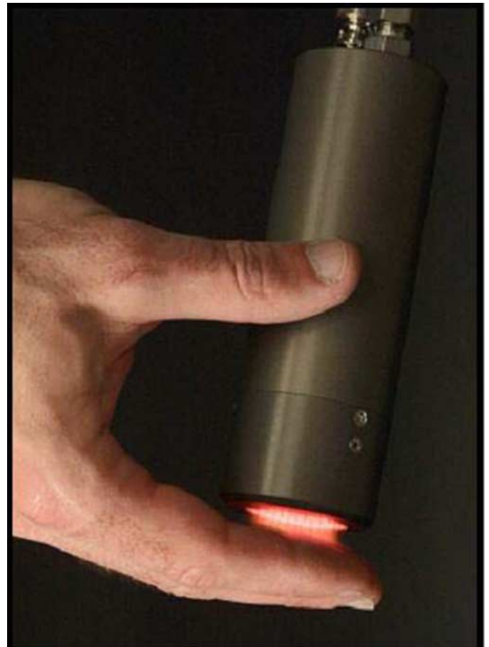
Fig. 1. Low-temperature, atmospheric pressure plasma (Courtesy of Surfx Technologies LLC).
